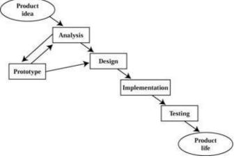
Figure 18–4: A sample of the rapid prototyping model **Assembling Reusable Components Model**
